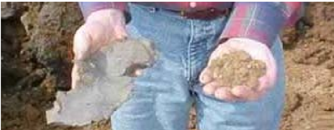
Figure 2: Comparing untreated plastic clay to lime-treated clay after initial mixing and mellowing
